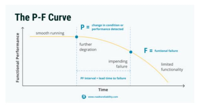
The curve shows that as a failure starts manifesting, the equipment deteriorates to the point at which it can possibly be detected (point "P"). If the failure is not detected and mitigated, it continues until a functional failure occurs (point "F"). The time range between P and F, commonly called the P-F interval, is the window of opportunity during which an inspection can possibly detect the imminent failure and give you time to address it.
